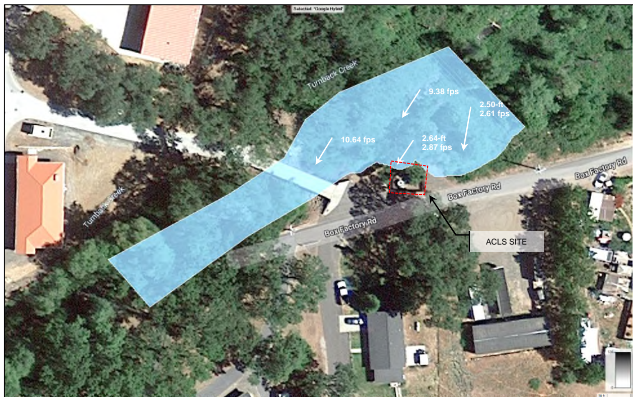
Figure 4. 1D model results of existing conditions with depths and velocities (100-yr event) noted.
